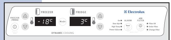
two digital displays on the left half of the control panel indicate the current temperatures of your freezer and fresh food compartments.
